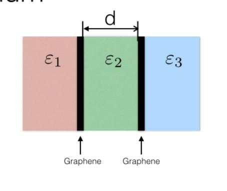
In a vacuum, the undoped bi-layer graphene system absorbs 4.4% of the EM wave, which is what we calculated with the transfer matrix method
